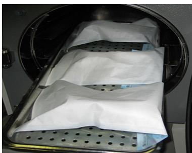
9. Select an autoclave cycle with a minimum sterilization temperature of 132° C (269° F) and that meets the exposure and dry time requirements stated below.
