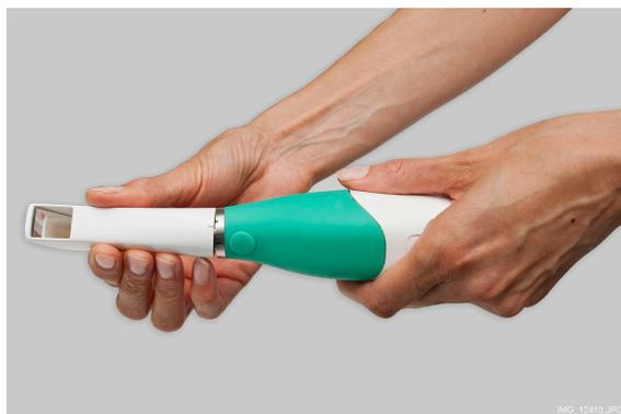
To reattach the tip, place the tip on the smaller notch on the scanner and turn it towards the larger notch on the tip until it locks in place.
